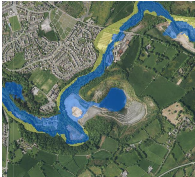
Figure 1.2 Extract of Development Advice Maps identifying extent of C2 flood area (in blue)
