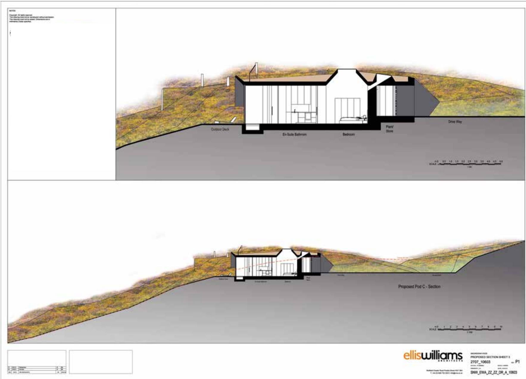
Figure-05 Typical Sections Embedded Into Topography
