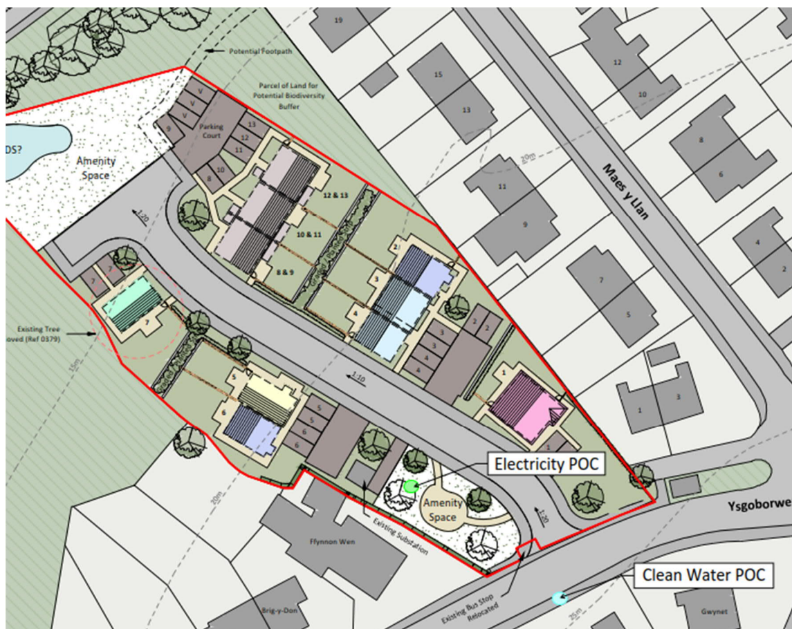
Figure 11.1 – Site Plan indicating position of points of connection
