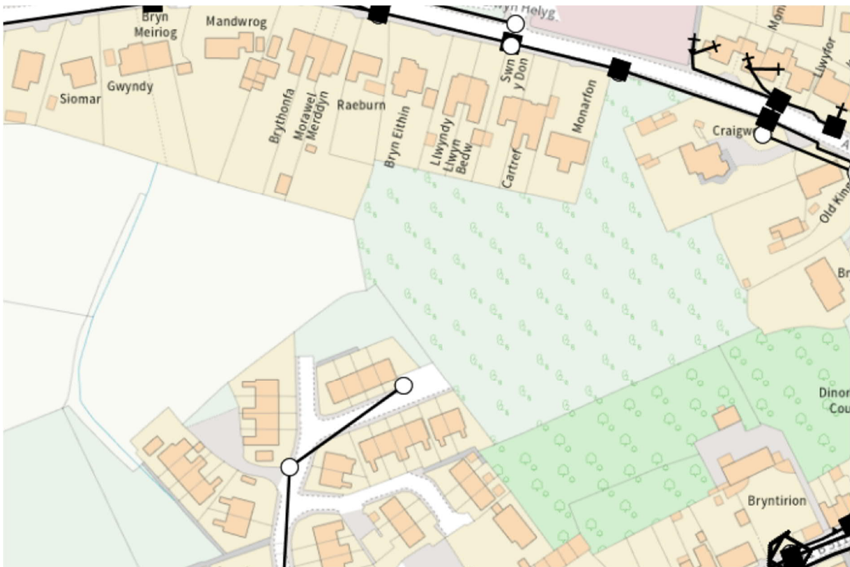
Figure 9.1 – Existing Openreach infrastructure
