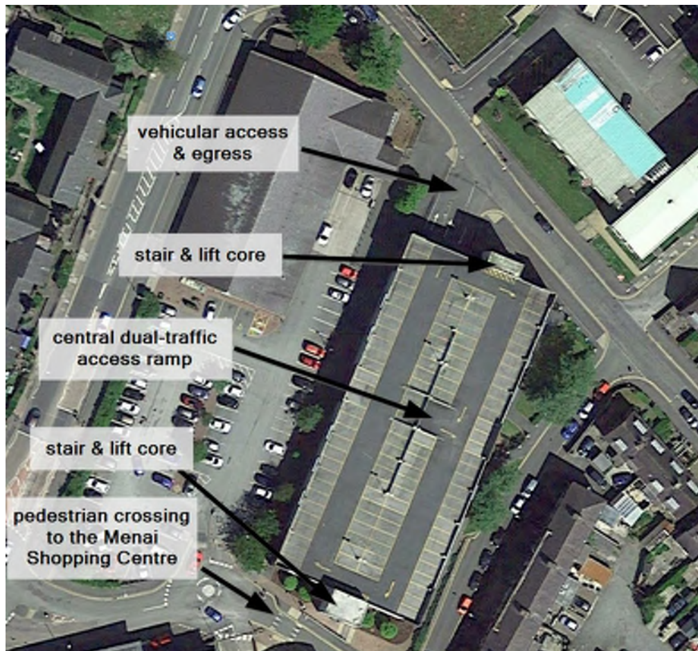
Aerial photo showing the parking space layout of the top floor & central ramp configuration.
