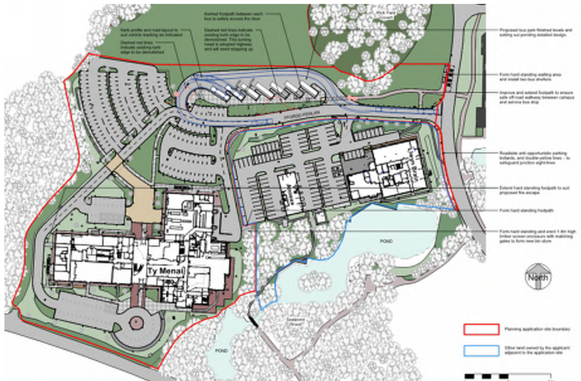
Siteplan illustrating the three existing buildings to be remodelled / refurbished, and the new proposed bus park
