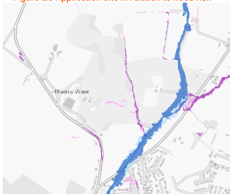
Figure 2.3 Application site in relation to flood risk
